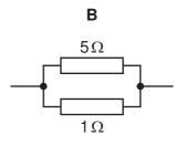
The total resistance is between  $1\Omega$  and  $5\Omega$ .
