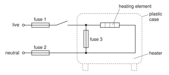
Which of the fuses are correctly placed?
