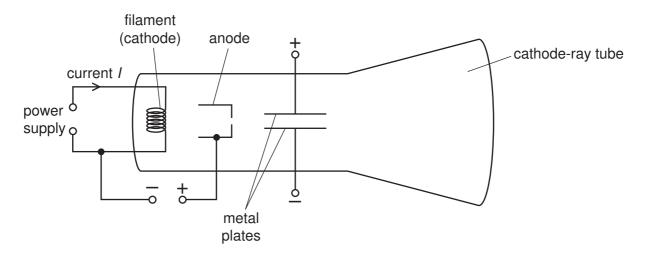
38 The diagram shows a cathode-ray tube used to produce cathode rays.
